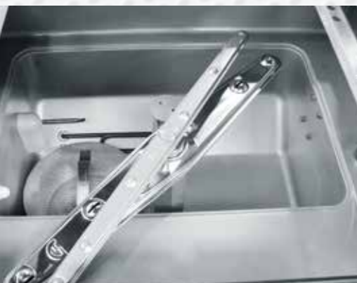
Tank with rounded edges and slanting bottom for the highest hygiene.
